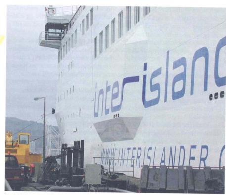
Shell blisters were fitted to widen the upper trailer deck.
