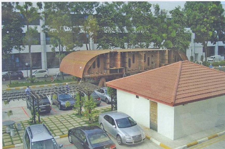
One of the new mid-ship sections: the first block (of twenty five) being moved during work in progress at Sembawang Shipyard (photo courtesy of Ray Newall).
